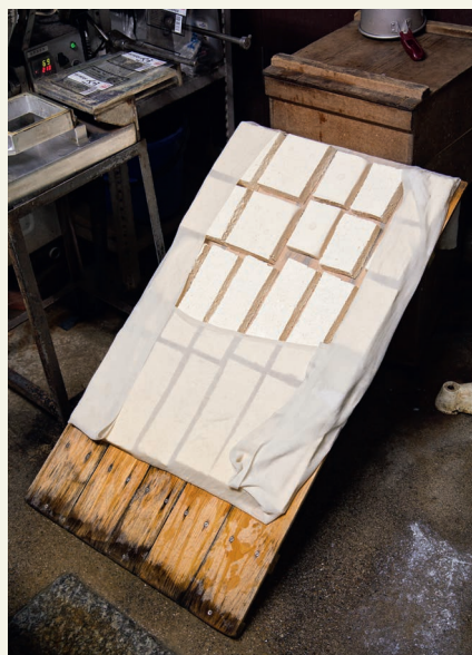
Using the inclined plane method to drain and firm up tofu in a manufacturing workshop in Japan.
