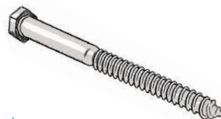
▲ LAG BOLT. Use for structural and de-mountable joints.
