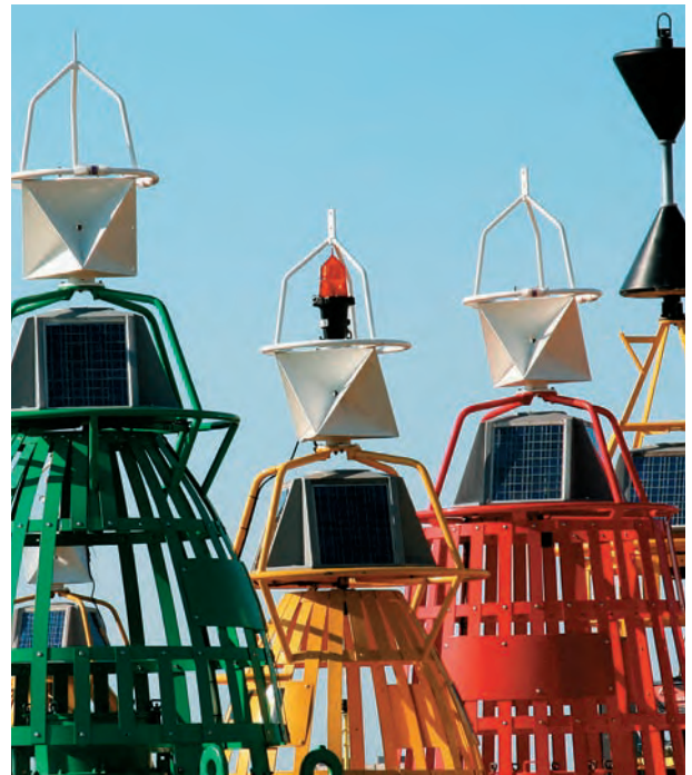
Buoy lights are a perfect use for a solar panel and battery. No other power source comes close to working as well and as cheaply for this application.
