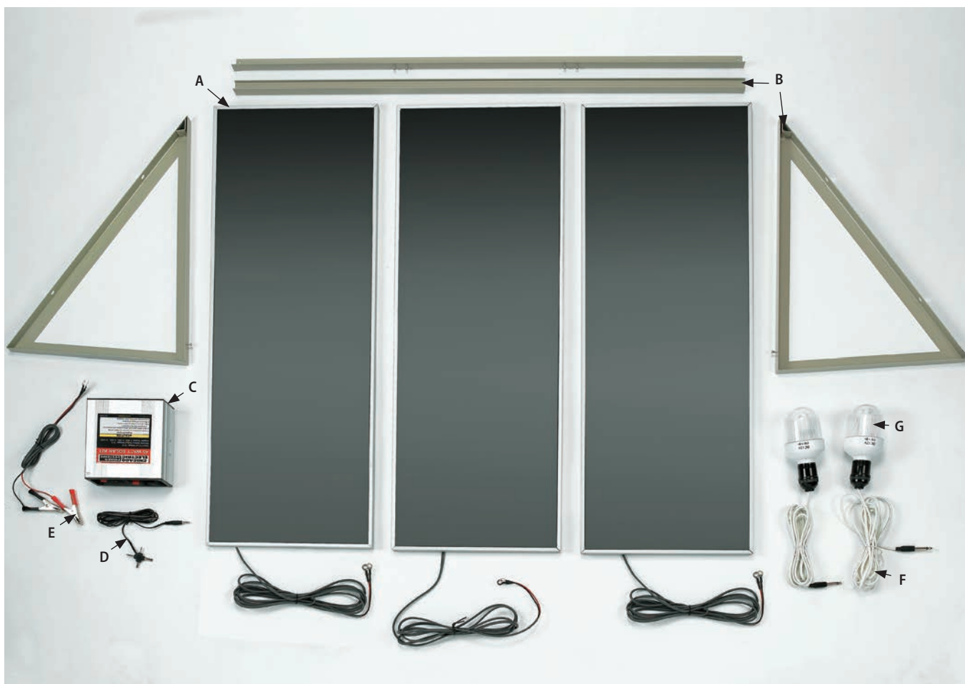
Parts of this solar light kit include: three 15-watt photovoltaic panels (A); snap-in mounting stand (B); regulator (C); multi-purpose adapter (D); battery connectors (E); light wires (F); 12-volt LED lights (G). A 12-volt battery is required but not included with the kit.
