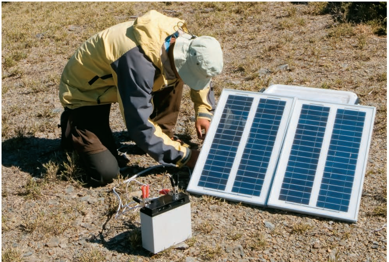
A solar panel and a small deep-cycle battery are a cleaner, quieter, and lighter source of temporary power for a trip away from the power grid.
