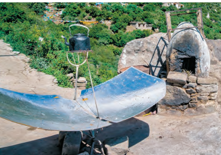
Heat fast, cook slow: A dish-type or parabolic solar cooker (left) creates a focused point of intense heat that can ignite paper in a matter of seconds or, more usefully, heat water or cook food relatively quickly. Cooking in a heat-trapping solar oven (right) is an all-day affair, but even homemade units can reach temperatures upwards of 300°F.
