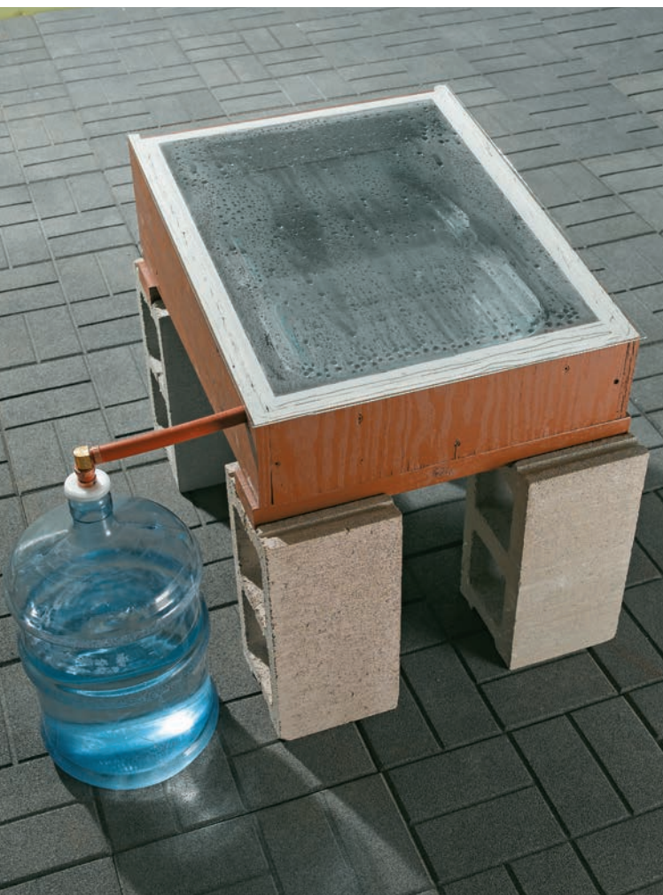
Purify and filter water: A solar still (left) works just fine to distill and purify water for modest consumption. A solar-powered pump (right) also may be used to filter water in off-the-grid locales.
