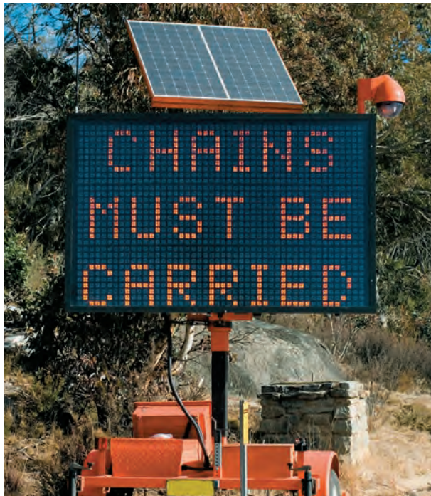
Solar power road signs are a common sight on highways. The light is plugged into a battery, which stores power produced by the PV panel. A charge controller keeps the battery from overcharging.
