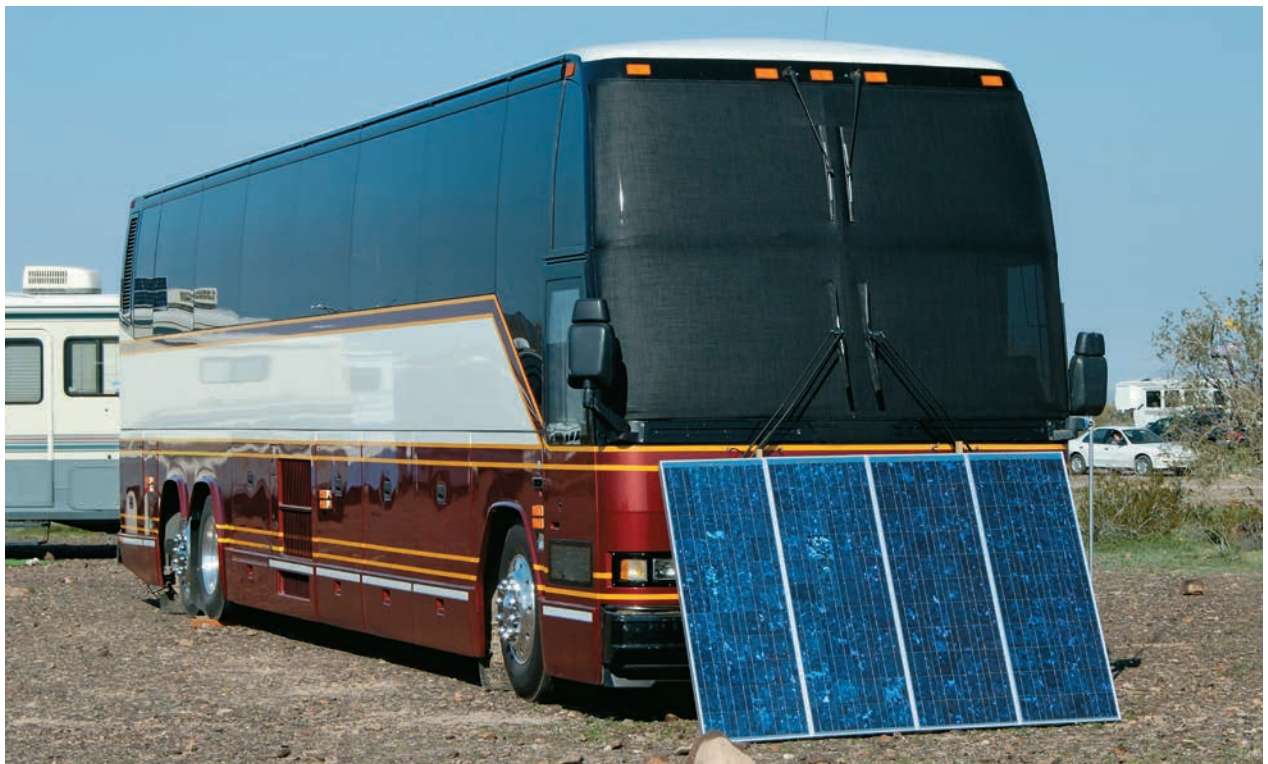
A camper van this size consumes as much energy as a small house, all of which would normally be generated by idling the motor. Although the large solar panels are a significant investment, they pay for themselves quickly in this desert campground, and they're also completely silent.
