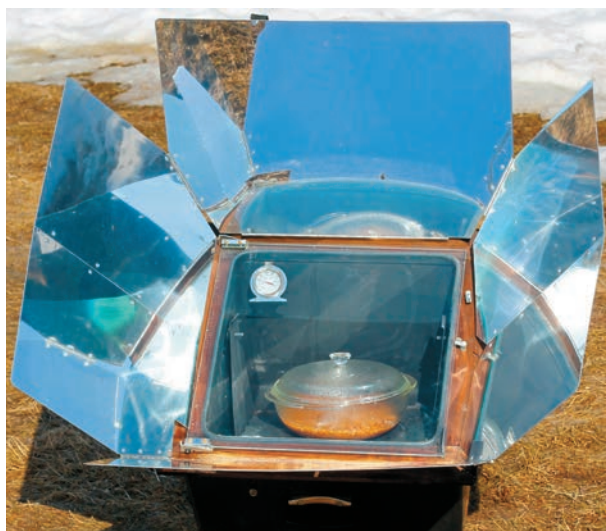
Heat fast, cook slow: A dish-type or parabolic solar cooker (left) creates a focused point of intense heat that can ignite paper in a matter of seconds or, more usefully, heat water or cook food relatively quickly. Cooking in a heat-trapping solar oven (right) is an all-day affair, but even homemade units can reach temperatures upwards of 300°F.
