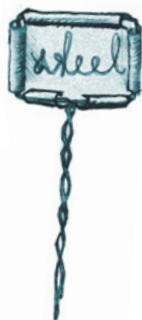
TWO-LEGGED WIRE PASSING THROUGH METAL BAND
