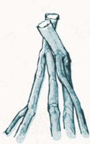
1 Tuteur frame formed with forked saplings joined at the top and splaying downward to facilitate assembly
